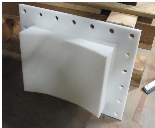
Figure 4 Sump Access Port sits Flush with Interior Manhole Wall
